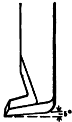
FIG. 4. — LEFT DIAMOND-POINT PLANER TOOL.
